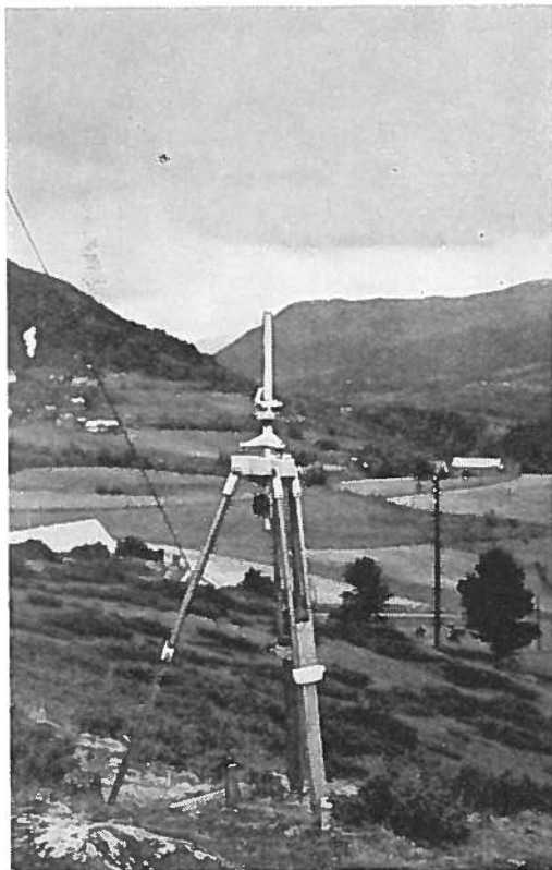
Fig. 10. View to the south. Field measurements at a point just below the absolute house. Azimuth mark is a break in the skyline; the pole in the foreground points just to the right of the mark. Stormy day in September 1955. (Photo G. G.)
